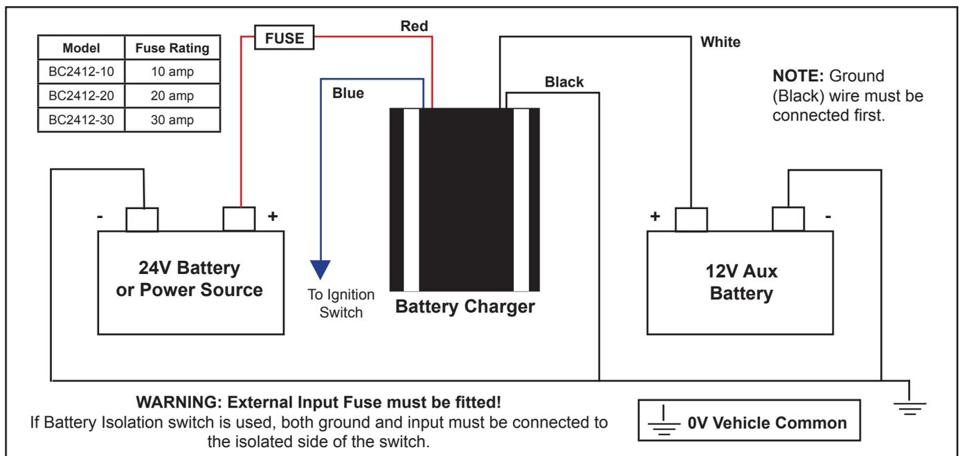
The battery charger is protected against over voltage, under voltage (during cranking of vehicle), over current (overload) and voltage spikes or surges. Under any of the above conditions the battery charger will shut down.
