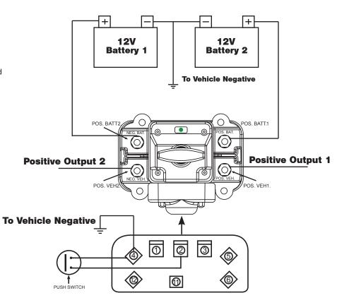
NOTE For Push Switch: Switch and Wiring must be capable of handling 50A Peak
