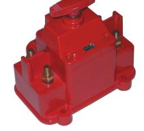
Using the base of the Master Switch as a guide mark and drill the four 8mm fixing holes. Secure in position with bolts, nuts and washers. The main battery leads need to be fitted with 10mm clearance eyelets and the auxiliary leads with 5mm eyelets. The use of petroleum jelly on the posts is recommended.
